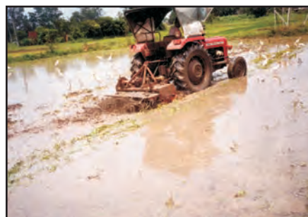
Field testing of tractor mounted rotavator for puddling of paddy fields
