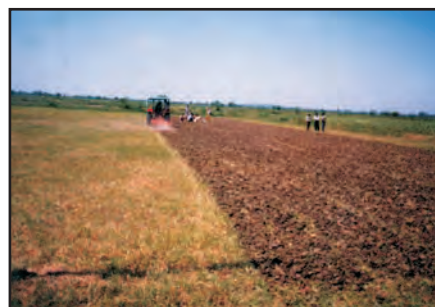
Field testing of tractor mounted rotavator for seed bed preparation (dry land)
