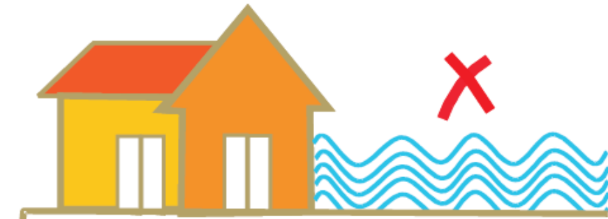
Construction at ground level –risk of inundation
